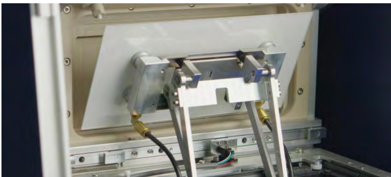
The highly sophisticated development chamber featured in the fully automated HPTLC PRO Module DEVELOPMENT allows for the active control of the gas phase.
