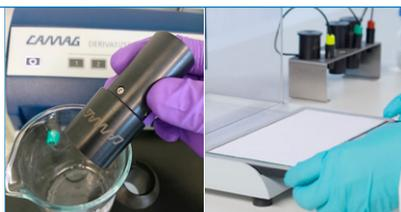
Empty the nozzle, if necessary, and insert a filter paper instead of a TLC/HPTLC plate and perform a spraying procedure with 2 mL of cleaning solution (level 6).
