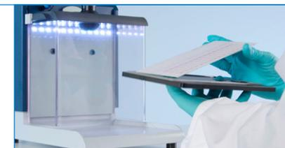
Lift the hood and remove plate.
