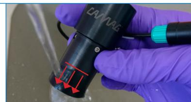
When necessary or when changing the reagent rinse the tip of the nozzle and the inside of the reagent container with (tap) water, ethanol or cleaning solution.
