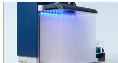
Wait until reagent has been sprayed, has settled on the plate, and the remaining reagent has been pumped out of the chamber.
