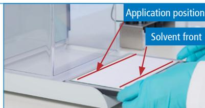
Insert the plate with the solvent front facing the front of the instrument and lower the hood.
