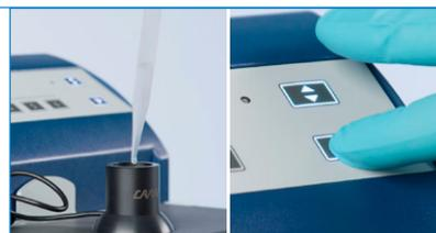
Fill the recommended volume of reagent into the nozzle and immediately start the spraying process.
