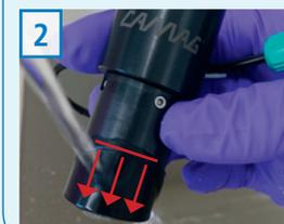
When necessary or when changing spraying reagent: **rinse the tip of the nozzle** and the inside of the reagent container with (tap) water, ethanol or cleaning solution.
