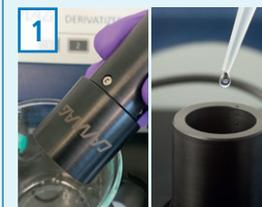
Empty the nozzle and spray 2 mL of cleaning solution before / after each spraying (level 6).
